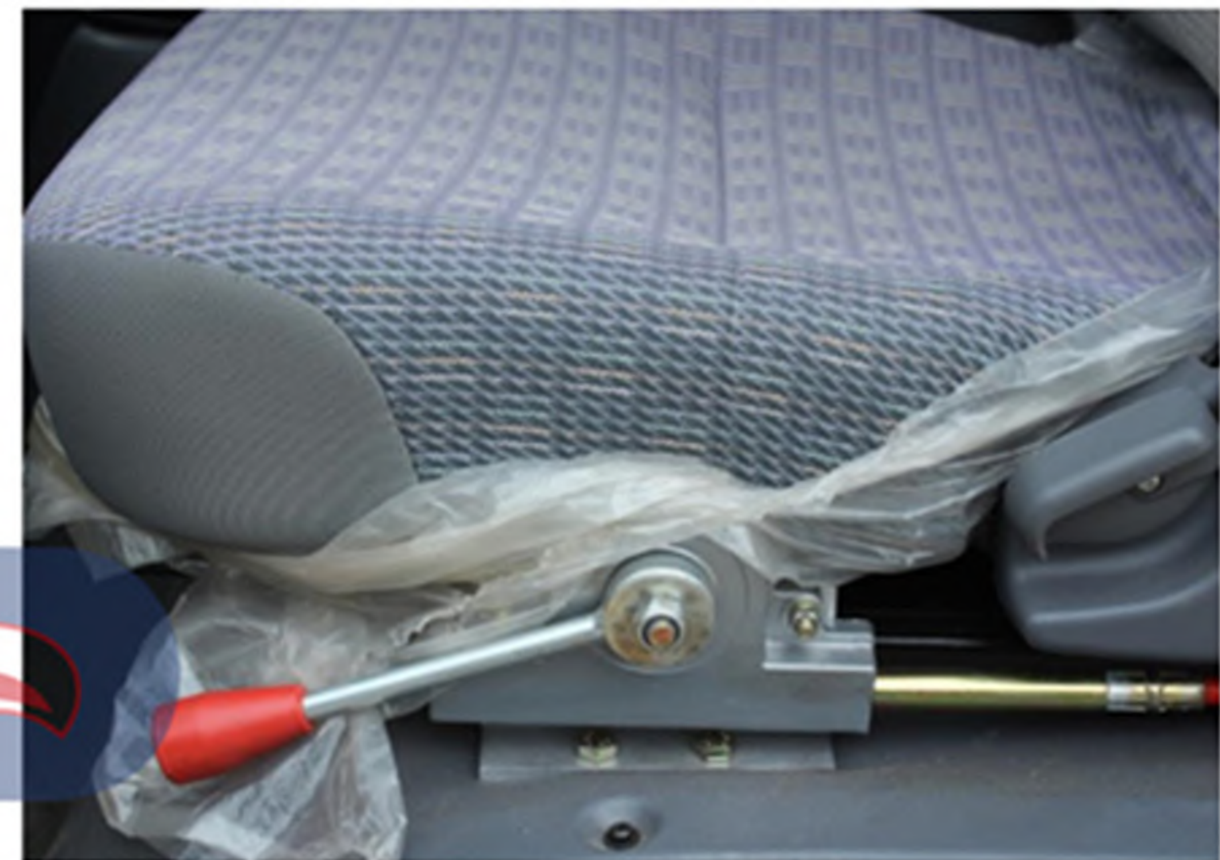
The Joystick at LOWER place The Man Lifter cannot work
